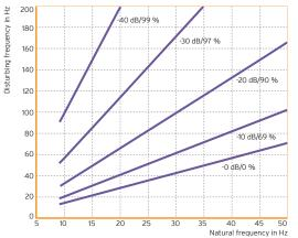
Reduction of the transmitted mechanical vibrations by implementation of an elastic bearing consisting of Sylodyn® NF
