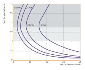
Static modulus of elasticity as a tangent modulus taken from the load deflection curve; dynamic modulus of elasticity due to sinusoidal excitation with a velocity level of 100 dBv re. 5·10-8 m/s; test according to DIN 53513
