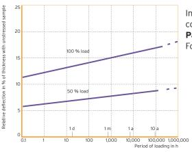
Increase in deformation under consistent loading
