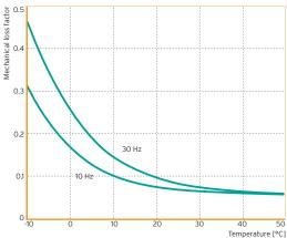
DMA-test (Dynamic Mechanical Analysis); tests within linear area of the load deflection curve, at low specific loads
