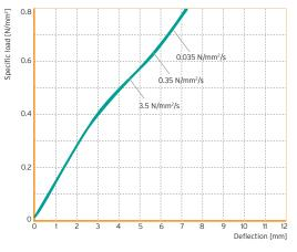
**Dependency on amplitude:** preload at static load limit; Form factor: g=3, thickness of material 25 mm
