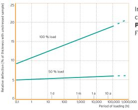
Increase in deformation under consistent loading
