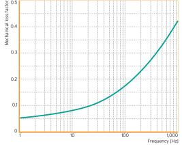
DMA-tests; mastercurve with a reference-temperature of 21 °C; tests within the linear area of the load deflection curve, at low specific loads
