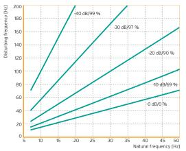
Reduction of the transmitted mechanical vibrations by implementation of an elastic bearing consisting of Sylodyn® ND
